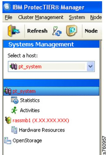
Figure 10. Faulty nodes displayed in red
